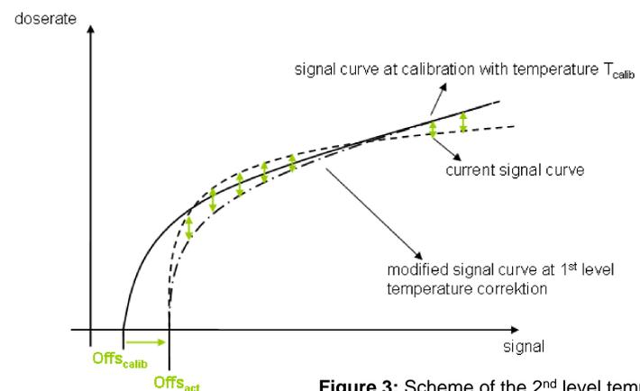
**Figure 3:** Scheme of the 2<sup>nd</sup> level temperature correction
