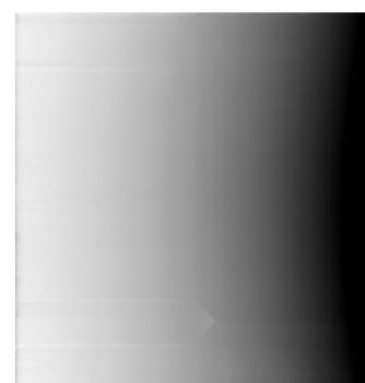
**Figure 4:** Wedge field after 2<sup>nd</sup> level temperature correction, taken by an over four-year-old panel
