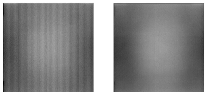
Single frames taken at PRF 200 – Left: without sync correction, Right: after applying the free-running Sync correction
